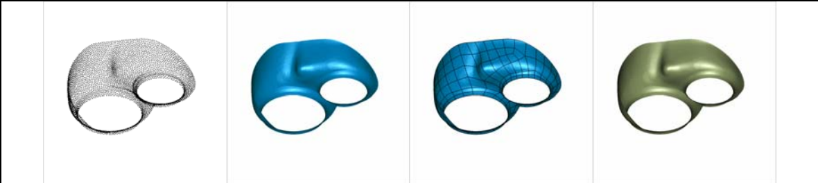
Series of images showing digital reconstruction of combustion bowl within Geomagic Studio software.
